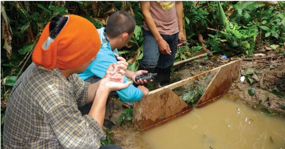
Figure 19: Placing the V-notch plank perpendicular to the streambed
